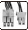
8P or 6P PCI-E connector (Some models offer 2-pin module detachable design): For graphic cards power.
